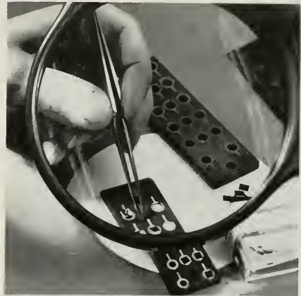
Germanium pellets, base tabs and emitter-collector materials being placed in an alloying jig.
